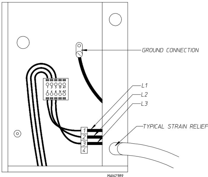
Providing local codes permit, power to a gas dryer or steam dryer can be made by the use of a flexible U.L. listed power cord or pigtail (wire size **must conform** to rating of dryer), or the dryer can be hard wired directly to the service breaker panel. In **ALL** cases, a strain relief **must be** installed where the wiring enters the dryer and service box area.
