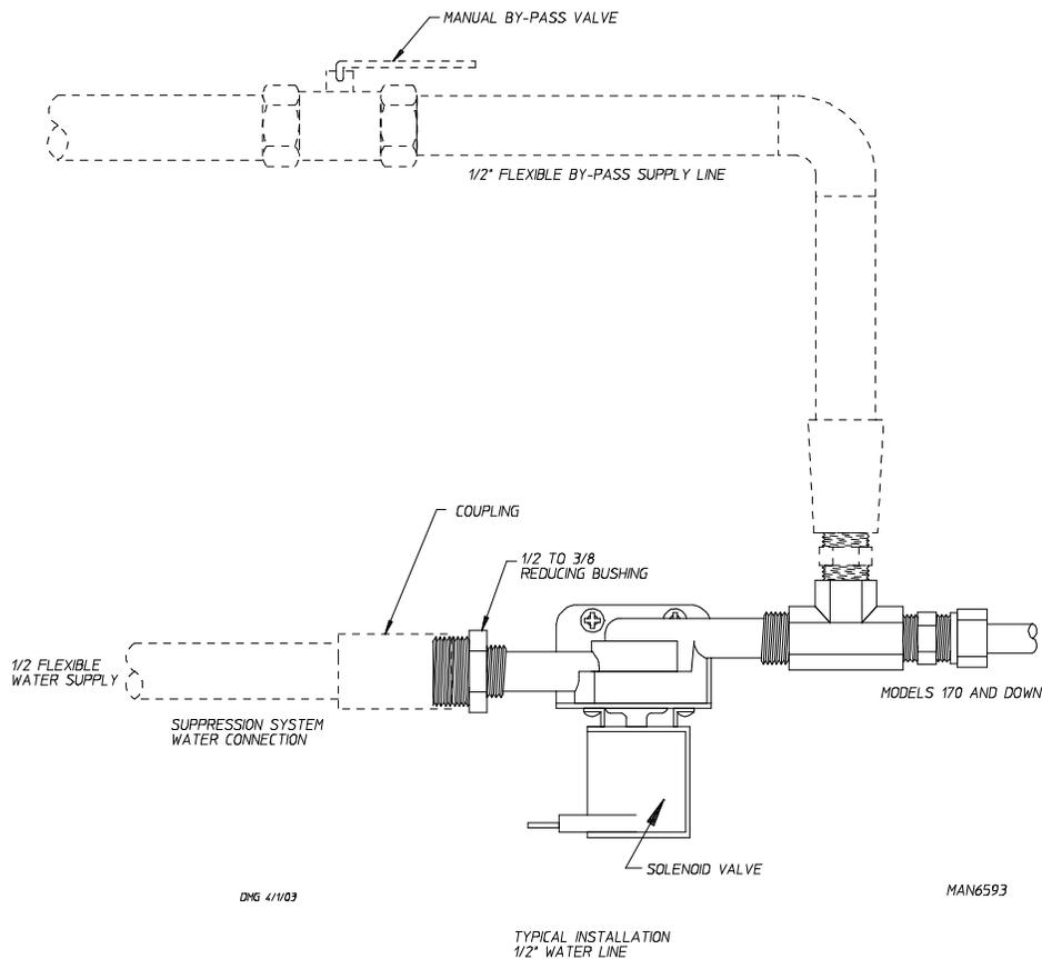
**WARNING:** If the water in the supply line or water solenoid valve freezes, the S.A.F.E. system will be INOPERATIVE!!
