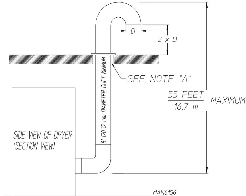
NOTE A: OPENING MUST BE TWO (2) INCHES (5.08 cm) LARGER THAN THE DUCT (ALL THE WAY AROUND) THE DUCT MUST BE CENTERED WITHIN THIS OPENING.
