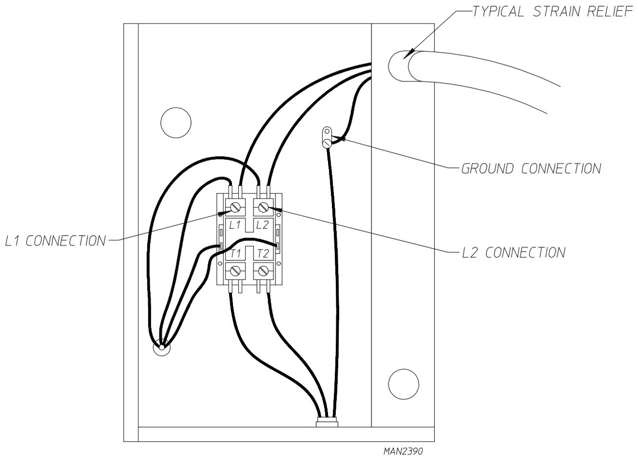
If local codes permit, power to the dryer can be made by the use of a flexible U.L. listed power cord or pigtail (wire size **must conform** to rating of dryer), or the dryer can be hard wired directly to the service breaker panel. In both cases, a strain relief **must be** installed where the wiring enters the dryer.
