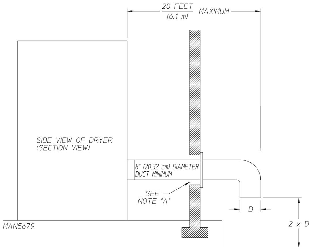
NOTE A: OPENING MUST BE 2-INCHES (5.08 cm) LARGER THAN THE DUCT (ALL THE WAY AROUND). THE DUCT MUST BE CENTERED WITHIN THIS OPENING.
